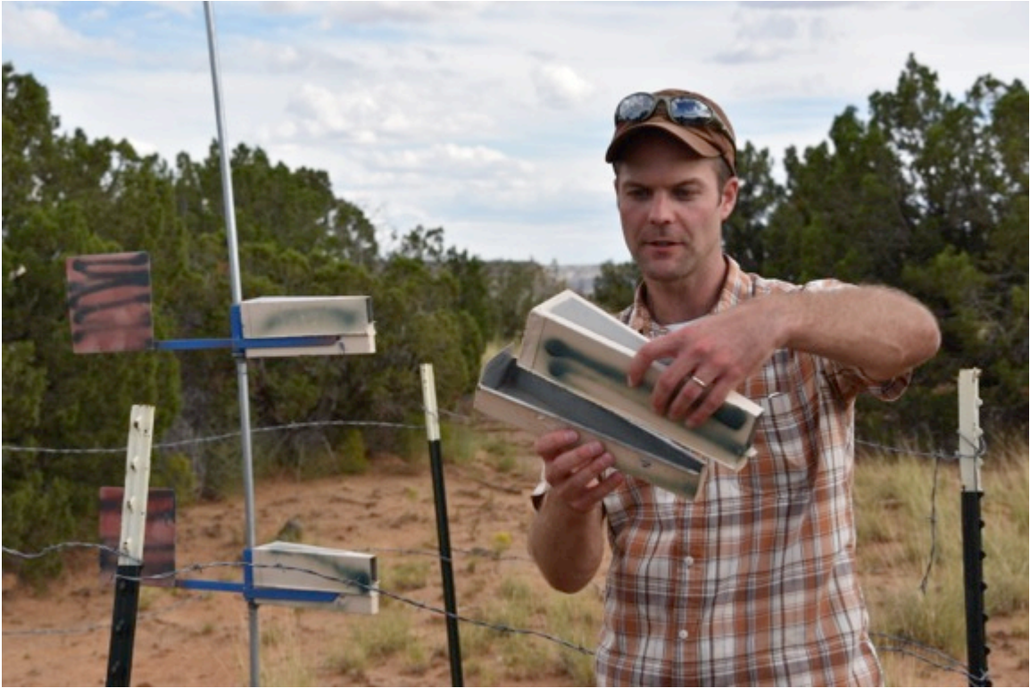
Dan Cadol (New Mexico Tech) checks his dust traps near the Jackpile-Paguate Mine on Laguna Pueblo
